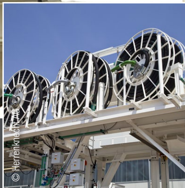
Hose reel during TBM build up for Herrenknecht "Karlsruhe" - Austria
