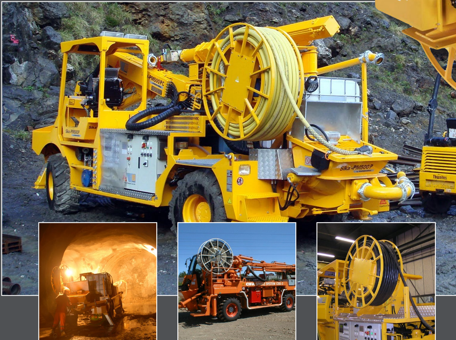
NAMI cable reel on shotcrete machine by Putzmeister
