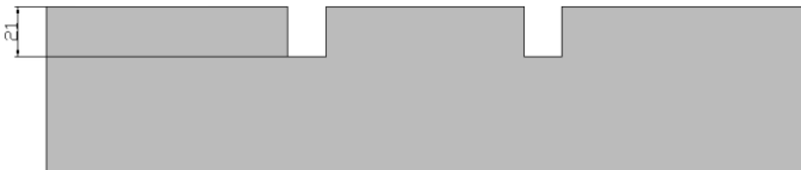
Figure 3.7: Grinding depth without floor coating
