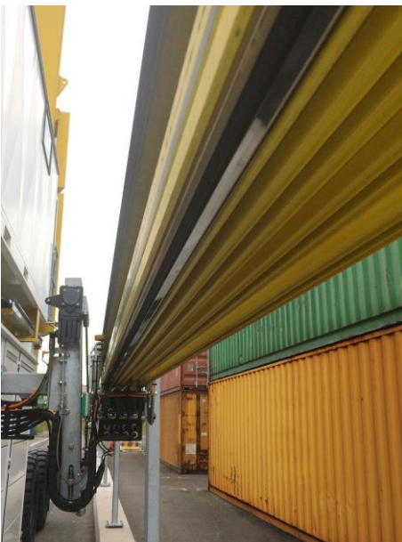
Caption: E-RTG solution: integrated energy and data transmission system ProfiDAT® with PE
