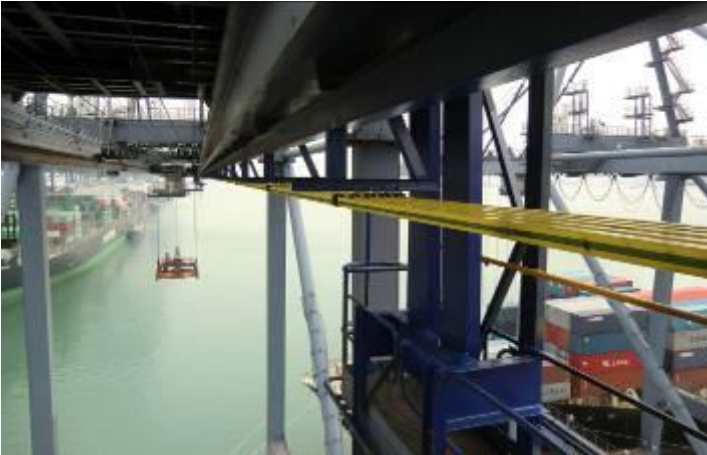
Caption: ProfiDAT® data transmission by Conductix-Wampfler is installed in parallel to the existing conductor rails on STS container cranes, or can also be installed in the PE as an integrated solution. The ProfiDAT® antenna moves inside the profile and is in contact with the transceiver via an Ethernet interface.
